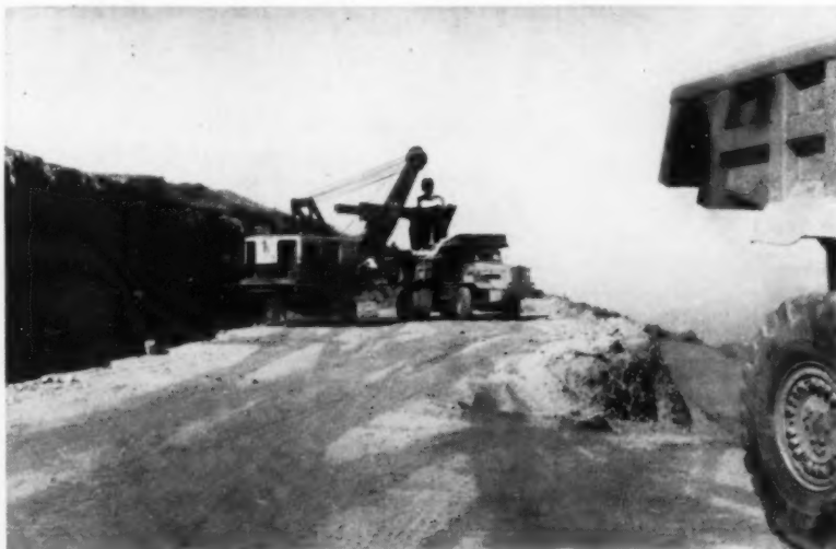
STRIPPING is not necessary since nickel mineralization extends to surface. Soft lateritic ore is loaded by 2½ cubic yard shovels into 30-ton dump trucks.
